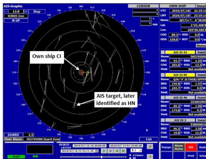
Figure 6: X-band radar screenshot with AIS overlay. (Source: MMD 35 and annotation by TSIB)
