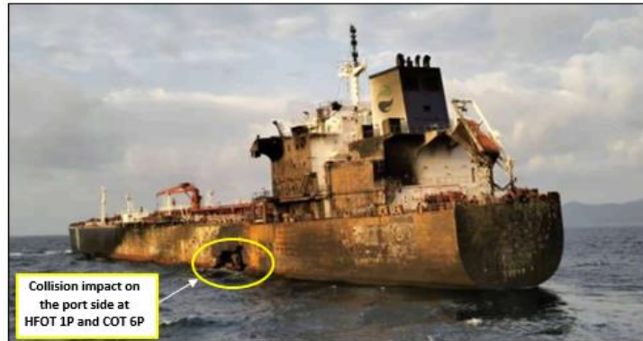
Figure 5: Image of the ship showing collision impact and subsequent fire damage. (Source: HN-Company and annotation by TSIB)
