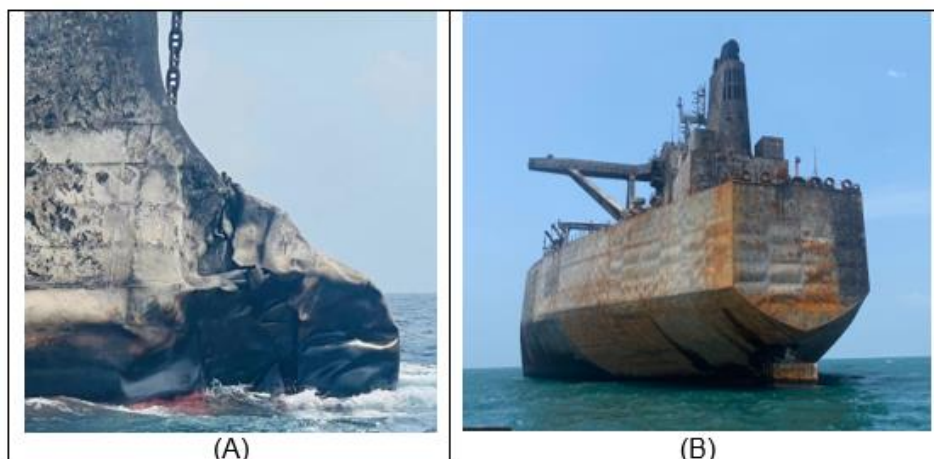
Figure 8: Images A and B of CI showing the damaged bow section (A) and fire damage of the hull and superstructure (B). (Source: CI-Company)
